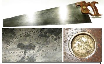
Photos above show a saw that is from 1865. A No. 7 saw that has a Henry Disston & Son etch but with a H. Disston eagle medallion. Thus here is a case in 1865 when they were using up the older H. Disston medallions on the newer Henry Disston & Son saws.
