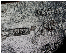
Above is axe by G.SHAU. To right is maker's mark stamped many times, but to the left it is stamped clearly.
