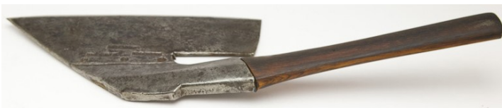
Above - Rohrbach axe showing the canted socket that angles the handle away from the wood being worked.
