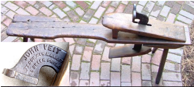
Shaving horse with iron jaw containing makers information.
