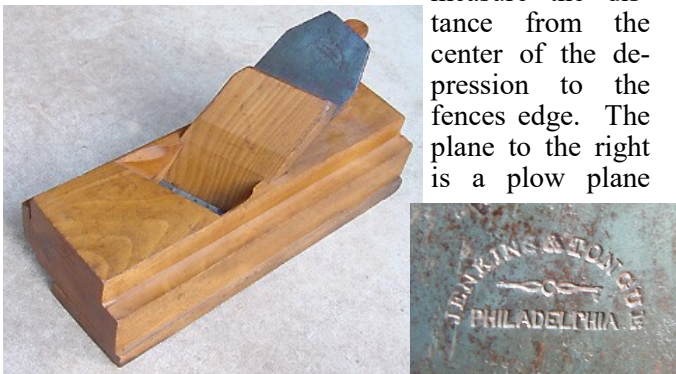
Large panel raiser with Philadelphia made iron.
