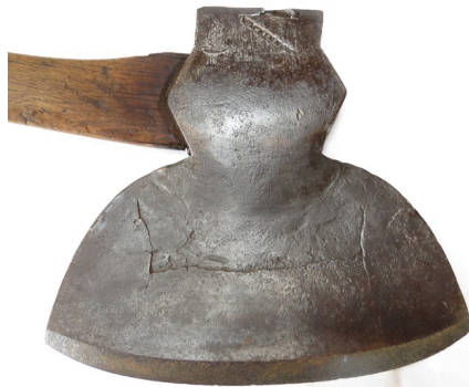
Broad Axe over-stamped with Wm. McKinnon mark for the repair done replacing the steel cutting edge.
