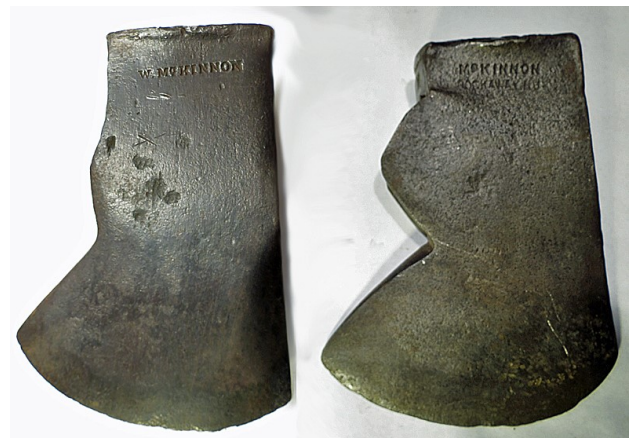
Comparison of two McKinnon axes. Left is earlier William McKinnon axe that follows closely the New Jersey pattern. On right is a later axe made by his son William that shows the full development of the Rockaway pattern.
