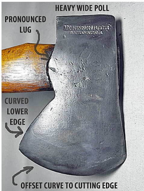
McKinnon Bros. axe showing the features of the Rockaway Pattern.
