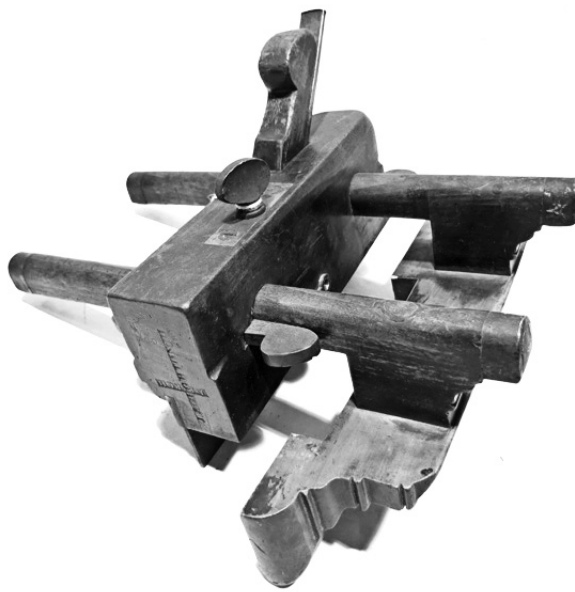
Left - wedge arm Plow plane by S.C.Cook, beech wood body with a boxwood fence.
