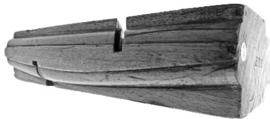
Above rear is two way coach plane with curved molding. Below this caption is bottom profile view of this plane. Above are two coach routers. Above right is small coach 1/4" groove plane. Maker of all planes is Mockridge & Francis. Chuck Granick's collection.
