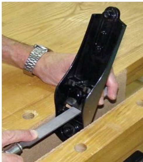
Gently clamping the plane in a wood vise angled back 15 degrees so you can hold the file level to file the front of the mouth.
