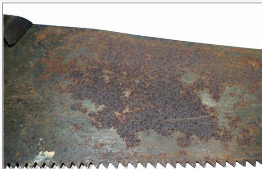
Above saw plate has rusting that is going to severely add pitting to the saw.
