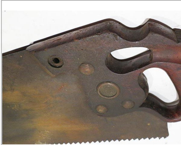
The saw above has a broke top horn and missing screw.
