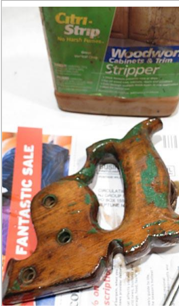
Above is handle with second application of stripper to remove the green paint.
