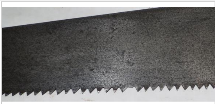
The above saw has a broken tooth, this will cause extra work when sharpening.
