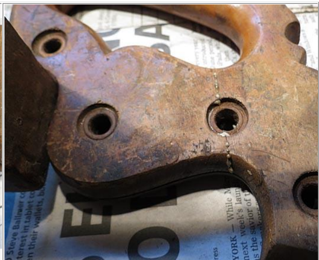
The crack is being glued and secured with a wood clamp. Glue can be seen oozing out of crack. This one held.
