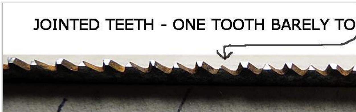
Above is initial jointing showing some teeth that were high and one tooth barely touched.
