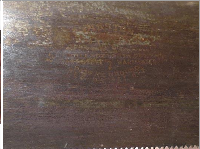
The saw plate above has a good strong etch under the accumulated tarnish.
