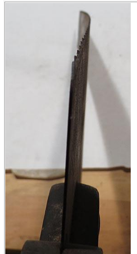
Sighting down the saw blade reveals a bent saw.
