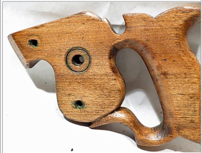
Top beech wood handle sanded and steel woolled. Bottom photo is the handle with light stain applied and two coats of Lacover French Polish finish
