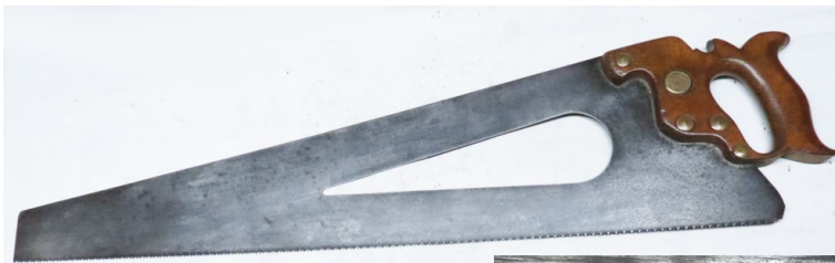
Above - Very unique Timber saw with cutout to reduce friction.
