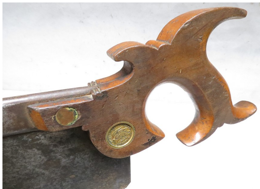
Above top - Richardson's special extra quality back saw. It is one of the most spectacular designs I have ever seen in a saw handle. Above bottom - A open handle back saw with the same all out handle design.
