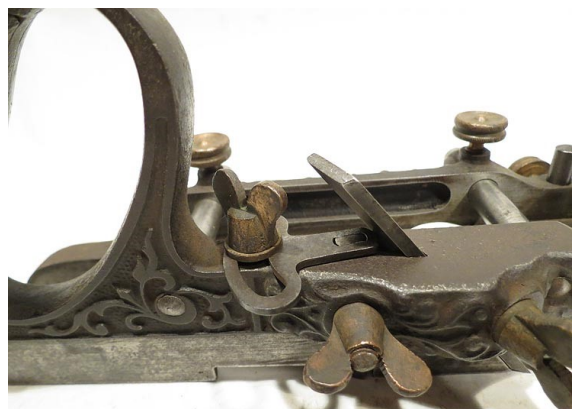
Above - Dorn patent plane showing swing out cutter with wingnut on top to lock in angle. Below - Right side of plane showing wingnut locking stem that comes up thru the body for the swing out cutter
