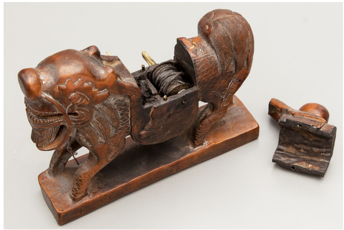
Above - A detailed carved horse sumitsubo with hidden inner line wheel and ink pot. Saddle removes to reveal inner workings. Photo courtesy of Jim Bode Tools.
