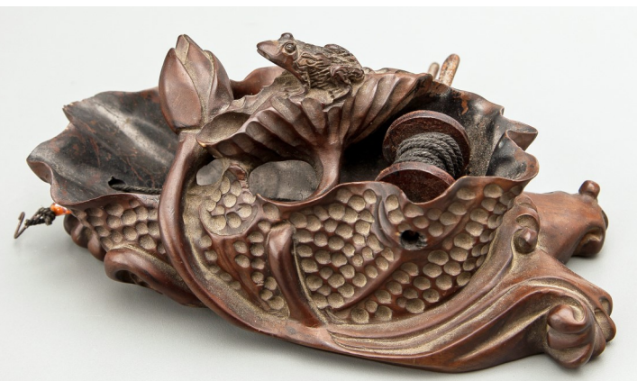
Above - An elaborate carved sumitsubo. It is unique in that it has one large carved depression containing both the line wheel and the ink pot. Photo courtesy of Jim Bode Tools.
