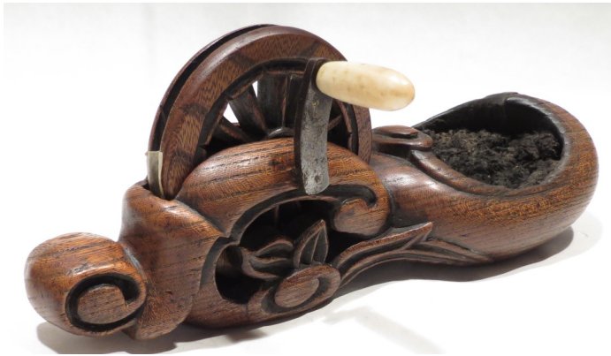
Above - A typical design of a sumitsubo with wheel for the cord, crank handle and ink pot.
