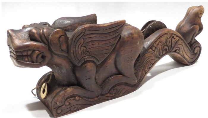
Above - A large ornate sumitsubo with dragon creature housing the inkpot. On the back a frog sits watching.
