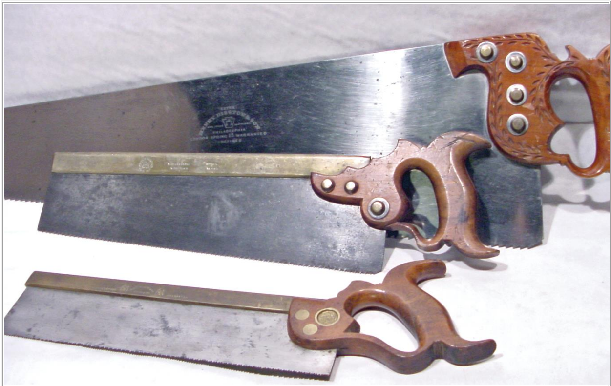
Three early Saws by the Disston Saw co. Top is a Disston & Son model No.12 with raised sawnuts in mint condition. Middle is a brass back saw with a tri-cove handle. Bottom is brass back Disston double eagle saw.
