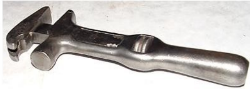
Hammer wrench having both patent dates for
