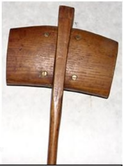
A Cooper's bung startle mallet has the head secured in a wedged mortise.
