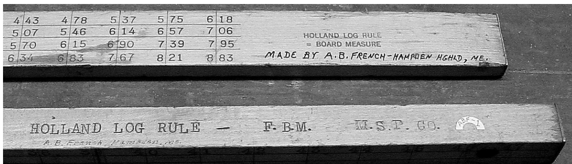
Two Holland log rules made by A.B. French. The top one is a three-foot long flat rectangular shape. It was made later in his career as shorter wood lengths were cut. The bottom rule has the initials M.S.P. CO. for the Maine Seaboard Paper Co. The initials F.B.M. stands for feet board measure.
