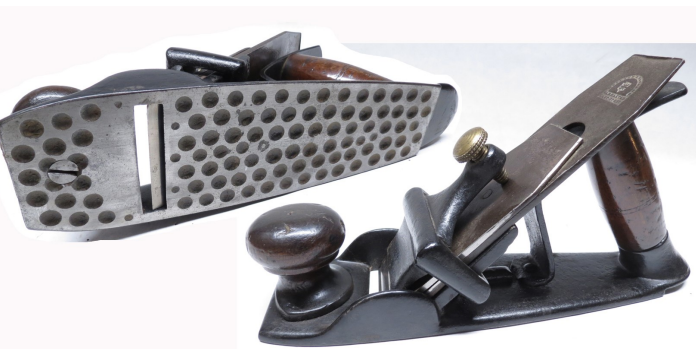
Above - Holly smooth plane with dimpled conical-shaped corrugations.
