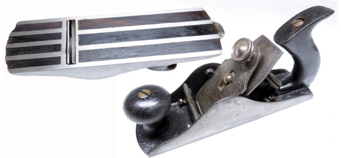
Above - Steers smoothing plane with dovetailed rosewood strips to reduce friction.
