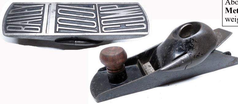
Above & right - Bailey Tool Co. block plane with their name cast into the sole as corrugations.
