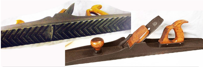
Above - Hazard Knowles , Colchester, Connecticut. Patent and date unknown. Knowles type jointer 27" long with Herring-bone pattern corrugated bottom. Photo courtesy of the D'Elia Antique Tool Museum.
