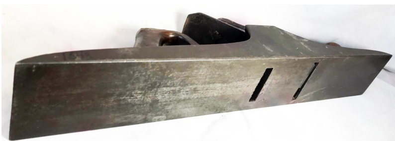
Above - Foster jointer plane with cut-out opening behind cutter for soap stone insert. Photo courtesy of the D'Elia Antique Tool Museum.
