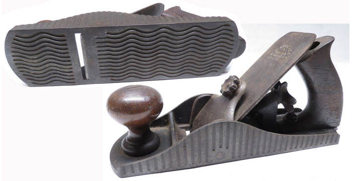
Above - Rodier plane with wavy corrugations on bottom.
