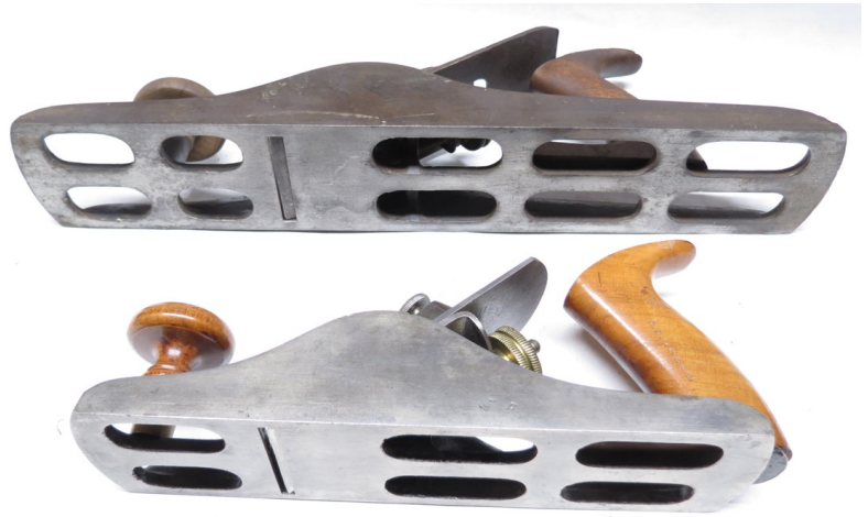
Above - Jack plane & Smoothing plane made by the Boston Metallic Plane Co. with open slots in the base to reduce weight and friction.
