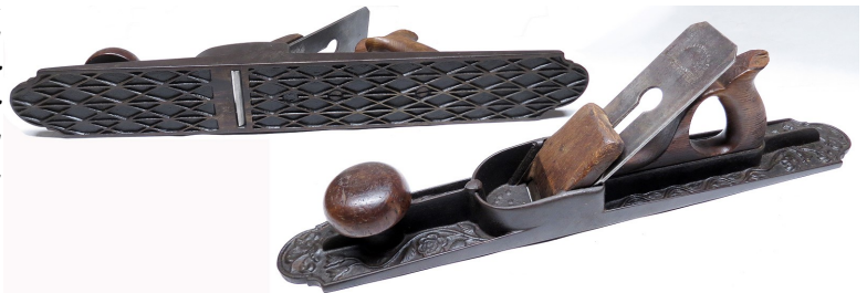
Above - Morris jointer plane with diamond shaped intersecting ribs on the bottom to reduce friction.
