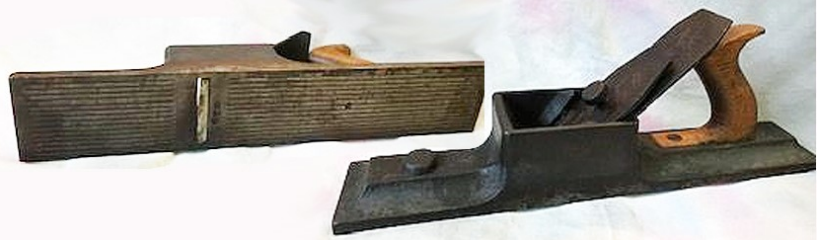
Above - Zoar fore plane -No known patent. Origin - Zoar, Ohio. Heavy cast iron plane with corrugations on the bottom. Photo courtesy of the D’Elia Antique Tool Museum.
