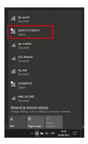
Once the serial number of the sensor is visible in the Wireless Network Connection list, select it and click "Connect". The Zenith60 and your device will be connected.
