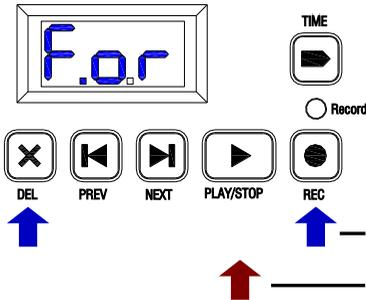
Format the memory device by pressing DEL+REC for 1 second. The display will show "For" and the dots will flash. The memory will be tested (display "tst") and the ICE-16 will automatically be set to either 24bit ("Hi") or 16bit ("Lo") mode depending on the memory quality.
