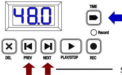
Check the sample rate the recorder is set to by pressing & holding TIME. The set sample rate will be displayed. For 16 channel recording this must be either 44.1 or 48kHz. Select the sample rate by continuing to hold TIME and pressing either PREV or NEXT. If you choose 88.2 or 96kHz then only channels 1-8 will be recorded.
