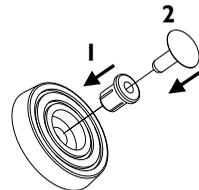
The feet can be fitted for desktop use or left un-fitted if rack mounted. Fit the feet according to the picture. To remove the feet later, prize out the central plastic rivet.
