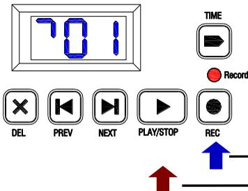
Press REC to start the first recording. The display will rotate segments and show the Song (or recording) number and the Record LED will be lit red. Press START/STOP to stop the recording or REC to stop and start the next one. Remaining time in minutes is displayed every 10 seconds (maximum 99 is displayed).
