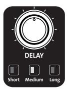
The Vocalist Live 3 provides 5 preset delay configurations. These are controlled by 3 buttons called Short, Medium and Long. Each button can be selected individually to get a different delay time. You can also select the Short and Medium buttons at the same time to get a medium-short delay or the Medium and Long buttons at the same time you get a medium-long delay. The delay times for the 5 settings are approximately 90ms to 750ms.
