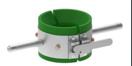
time. Pioneer versatile stabbing guides are designed and manufactured using aluminum shells and polyurethane inserts, in various sizes for several connection designs. The well-designed latching mechanism provides for quick engage and disengagement of the stabbing guide to increase safety and efficiency during use.
