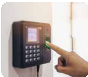
Access Control System
