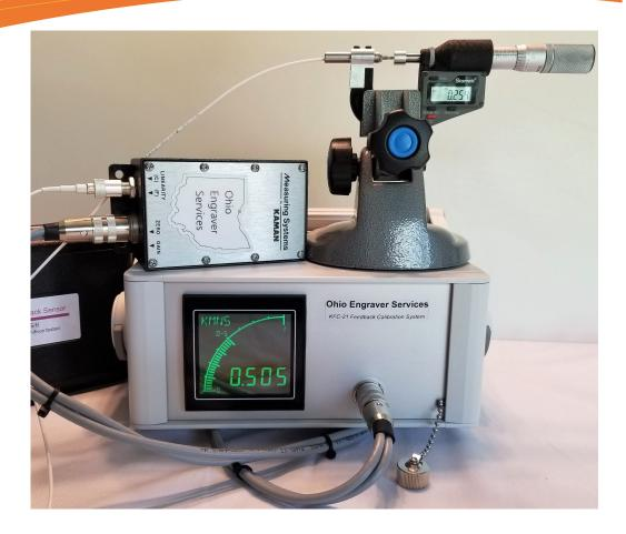
Vision Engraving heads with feedback control systems are renowned for excellent engraving quality, consistency, and flexibility to cover a wide range of screen/angle/diamond combinations. But problems caused by dirty or damaged Kaman feedback sensor can be disastrous and very expensive. Common Kaman sensor failure symptoms include, extremely poor cell shape, cell instability (ringing or drift) and even cause catastrophic damage to the engraving head, amplifier, or power supply.
