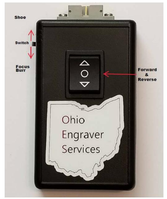
9v battery powered, this is the perfect troubleshooting tool for M820, Gravostar HS, Spectrum and Prism Prime engravers. Convenient motor selection switch allows to control Shoe motor or Focus & Burr Cutter motors. Forward & Reverse direction rocker switch for precision control and keyway placement.
