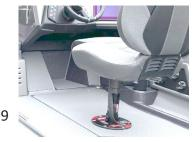
7. Tighten both locking rail bolts. Locking Rail should be able to move without sticking.
