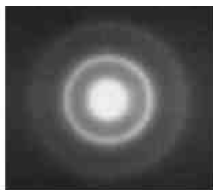
Fig. 2.13: Electron diffraction pattern from nickel crystal
