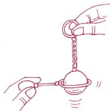
Fig. 14.5 Ball and ring experiment to demonstrate thermal expansion
