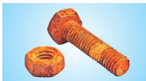
Fig. 4.9: Rusty nuts and bolts of iron
