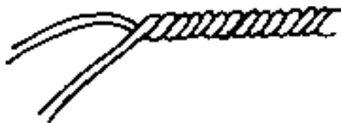
Fig. 23.4: Two Ply yarn
