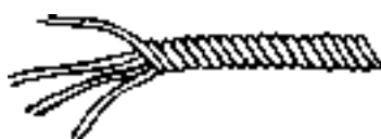
Fig. 23.6 : Four Ply yarn
