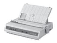
Fig. 1.13 Dot Matrix Printer
