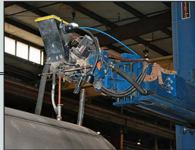
Three PLC Submerged ARC Welding Systems with 3-Axis Motion Control and a direct view vision system to control seam welding and provide real time inspection at 10x to 25x magnification
