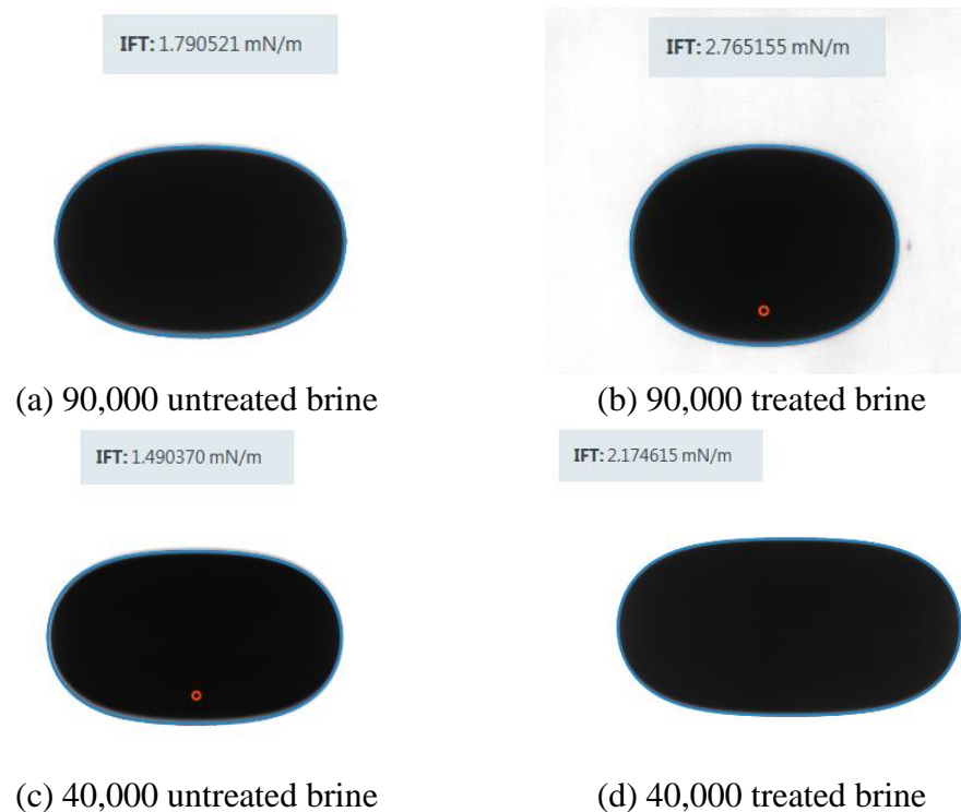
Figure 8. The IFT between oil and brine (a) 90,000ppm brine; (b) 90,000ppm treated brine; (c) 40,000ppm brine; (d) 40,000ppm treated brine;
