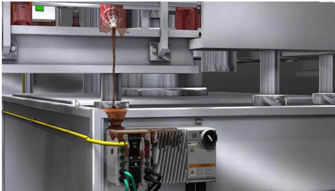
Some on-machine solutions are designed to withstand grimy, harsh environments and can be washed down with water.
