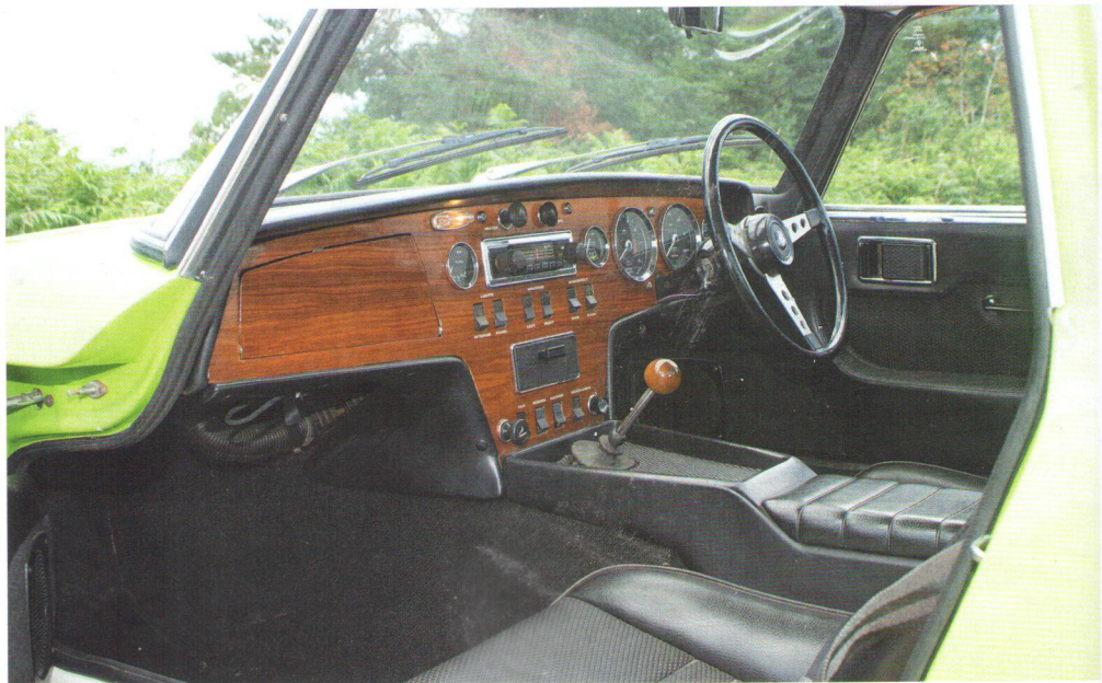
Dashboard survived the crash unscathed and was carried over to the new bodyshell.
