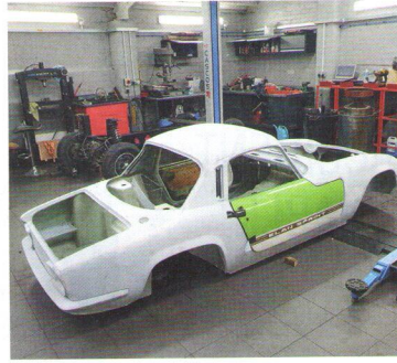
Original doors lined up in new 'shell.
