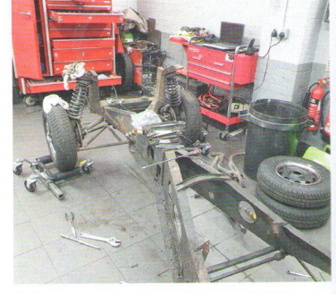
Stripped back to the bare chassis.
