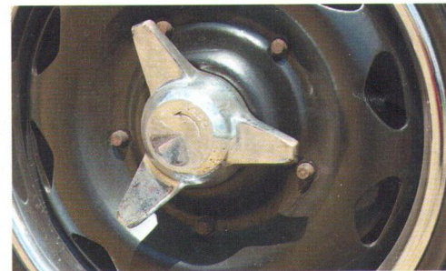
Lotus steel wheels fitted with knock-off spinners.
