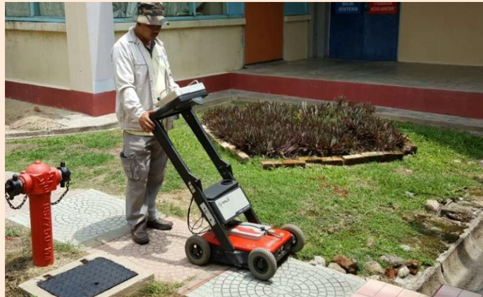
The use of GPR Equipment at Site
