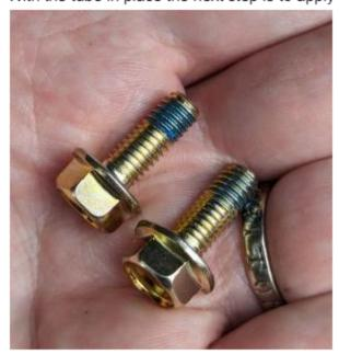
The thread lock compound should be placed at the thread end of the bolt. Use only medium strength thread lock as supplied in the kit. Never use permanent or red thread lock.
