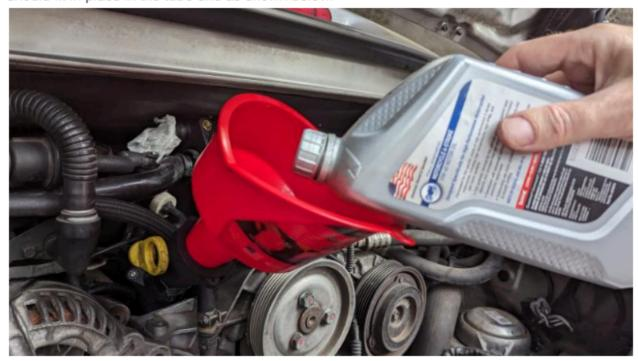
It is not recommended to fill oil without using a funnel; spilled oil can drop directly onto the serpentine belt underneath and will cause slippage.
