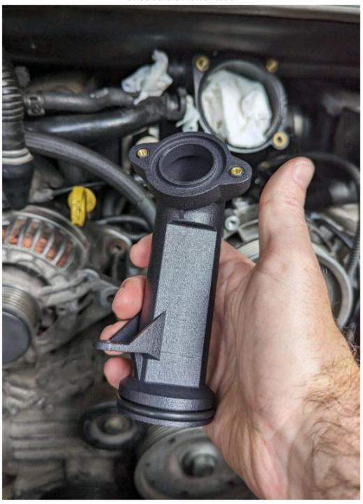
Check the tube for any defects as outlined in warranty section (3). Confirm the main crankcase O-ring is in place. If it is not; carefully stretch and fit it onto the tube as shown in the above image. A little grease or engine oil is acceptable to help it slip onto the tube. The red plastic plug may also be pre-installed from the kit.
