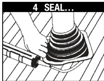
Apply sealant between base and roof.
