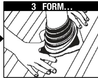
Press Master Flash down, bending it to conform to roof profile or roof irregularities. A blunt tool will help press flashing into tight roof angles.
