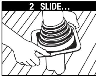
Slide Master Flash down over pipe (A non-petroleum base lubricant will ease installation).
