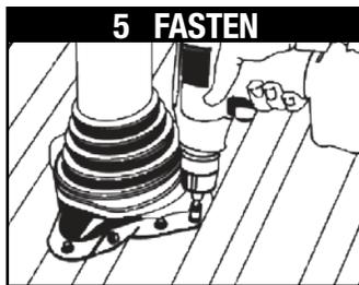
Use fasteners to complete sealing. For UPC installation, fastener spooning may not exceed 1-1/2" (38 mm).
