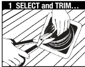
Choose appropriate Master Flash with opening at least 20% smaller than pipe diameter. If necessary trim opening to 20% smaller than pipe diameter.
