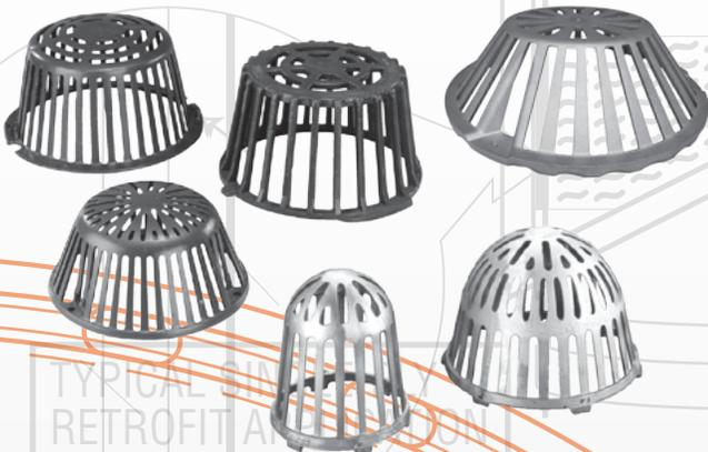
These rigid, durable strainer domes are fabricated of cast aluminum or cast iron. Some units are attached by twist n lock action. Others are attached by the bolt down means and are best suited for use on school roofs and other applications where security of drain openings is a concern. Selected models are available in bronze metal. Available Sizes 5", 8", 10", 10" Low Profile and 12".
