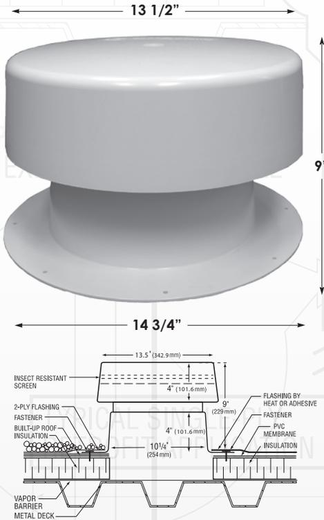
Pre-vent design provides venting capacity to accommodate 327 sq. feet of floor. The Pre-Vent is UV stabilized to help reduce any deterioration and fading from the sun. To install the Pre-Vent properly it has been designed with pre-drilled holes in the flange to attach the Pre-Vent to the deck.
