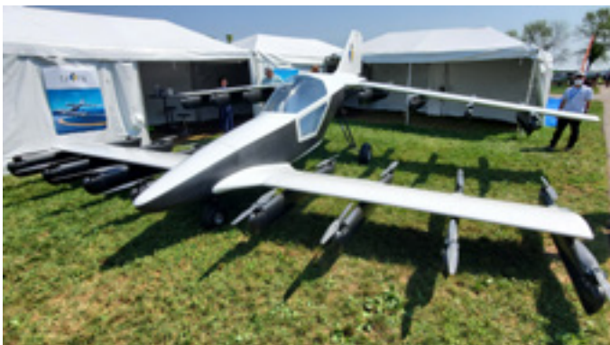
Tokyo-based teTra displayed its Mk-4 eVTOL with 32 lift propellers as a follow-on to its Mk-3 entry in the GoFly Prize competition.
