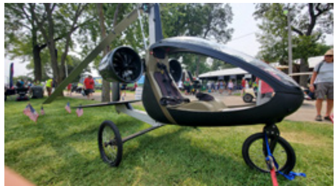
Luminati displayed an electric gyrocopter testbed used to demonstrate its twin 40-kW nacelle electric fans.
