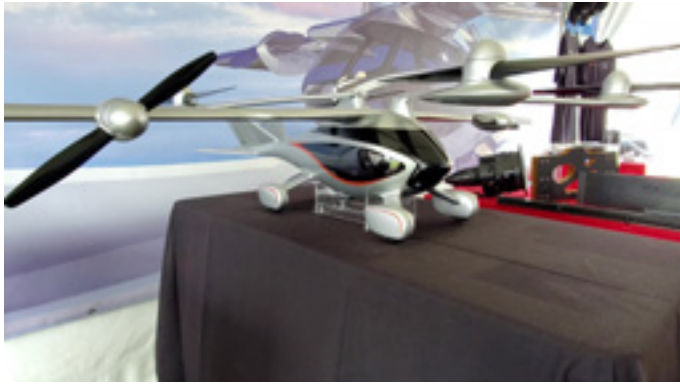
Model of NFT's ASKA eVTOL flying car, which folds its four arms and two wings, each supporting an electric propeller.
