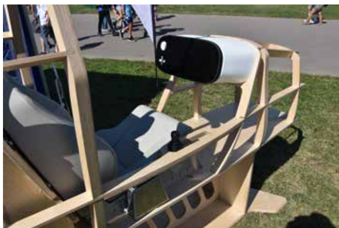
teTra Aviation displayed a cabin mockup of its Mk-5 eVTOL kit aircraft to get visitor input.
