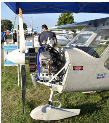
Chris Erwin's Merlin ultralight aircraft with his Aeromarine Merlin Parallel Hybrid Drive.
