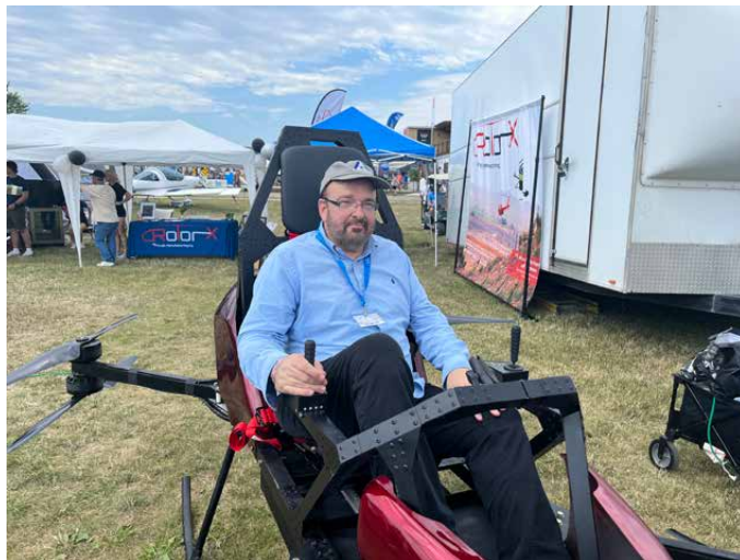
Rotor X CEO Don Shaw sits in the new Dragon single-seat ultralight eVTOL. The arms fold inward for transport and storage.
