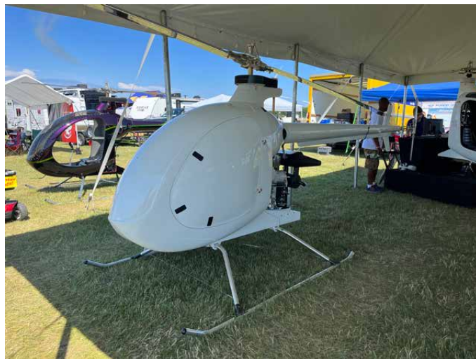
Composite-FX brought six variants of its single-seat kit helicopters, including this autonomous, uncrewed Mosquito.
