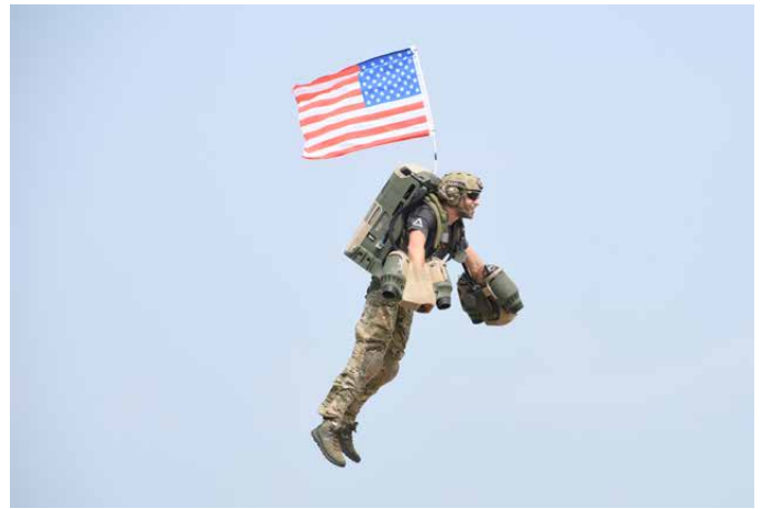
Gravity Industries inventor and CEO Richard Browning gave stunning demonstrations of his latest jet suit with five turbojet engines.
