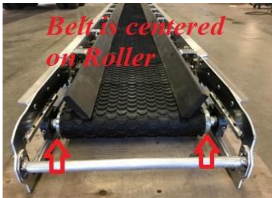
This belt is tracking correctly.
