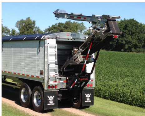
Conveyor is Raised all the way UP, when Folding & Unfolding.
