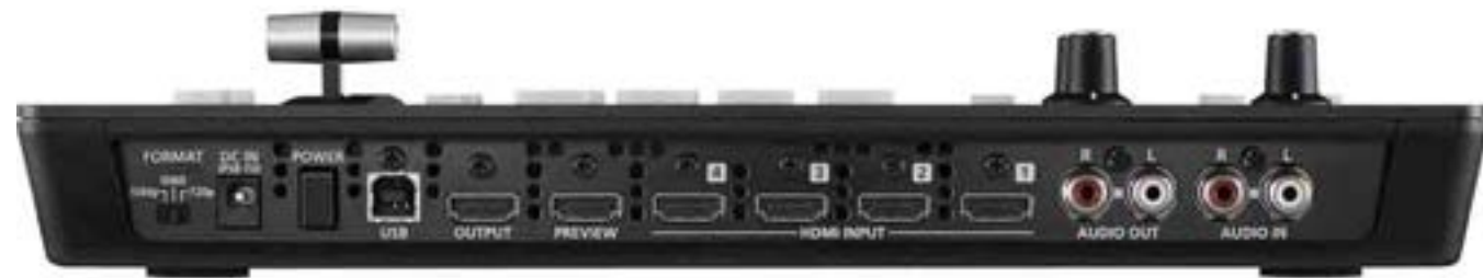
A quick glance at the back of the Roland V-1HD, reveals how simple it is to connect 4 HDMI outputs from cameras, a USB computer connection, along with audio I/O and HDMI connections to preview and final output monitors.
