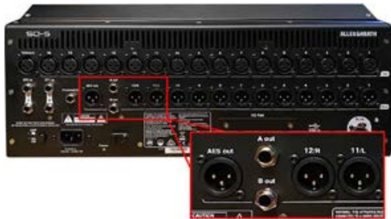
This mixer includes two balanced XLR outputs, two 1/4-inch balanced TRS outputs, and an AES XLR output.
