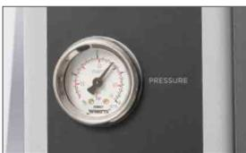
Gauge to display the pressure of the upper roller
