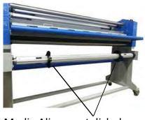
Media Alignment disks keep supply rolls from telescoping
