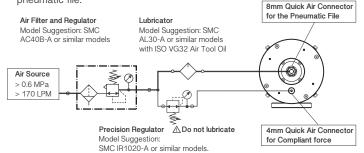
Check the CENTER POINT (\*1) first; giving 0.1MPa pressure to the compliant force connector while the pneumatic file is turning off. Make sure the pneumatic file is able to return to the CENTER POINT as shown as the illustration below. Please contact your supplier if it couldn't return to or is not on the CENTER POINT.
