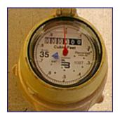
The meter shown below, also cubic feet, is good example of a situation where the final number has already "turned over". The correct reading on this meter is: 2425.92 cubic feet. On most meters, the final digit will turn over once the big sweep hand has passed the 0.6 mark.
