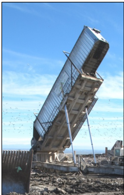
Unloading a transfer trailer at Altamont Landfill.
