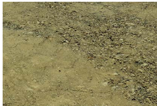
Close-up of ET cover subsurface soil. Largest fragments are approximately 2 to 3 inches
