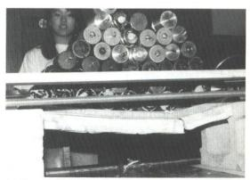
This bridge worked—barely. The students who built this one now have a much better appreciation for crack tip propogation, speed, and critical crack length.
